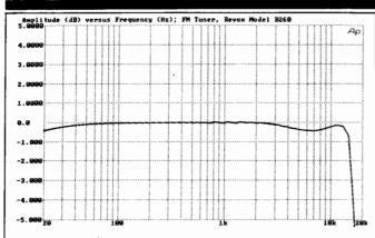
Fig. 5—Frequency response. Note vertical scale of 1 dB/div.
