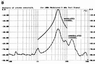
Fig. 6—Separation and crosstalk components for a 5-kHz modulating signal, plus subcarrier and sideband components, for wide (A) and narrow (B) i.f. modes.
