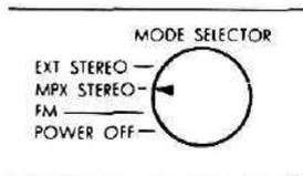
Fig. 5—MODE SELECTOR in the MPX STEREO position.
