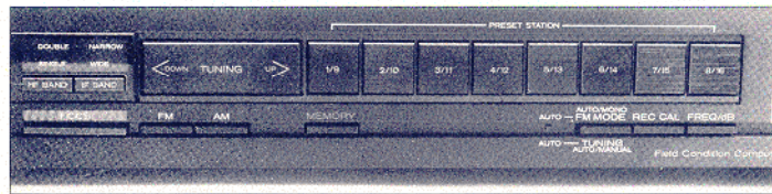
The PT5500's features include 16 presets and the FCCS circuit which optimises bandwidth settings according to the reception conditions
